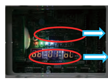
① Debugging button Three dual 8 nixie tubes display debugging status with high readability
